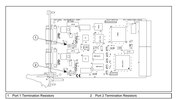
**Figure C-5.** Location of Termination Resistors on a PXI-8460
